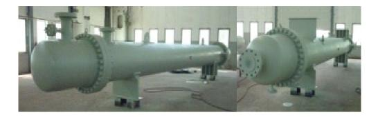
Project Sourgas: 24 Pulsation dampers acc. ASME VIII div.1 for HIC application, design pressure up to 270 barg
