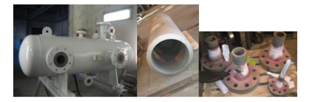
**Project North Stream:** Natural Gas conditioning plant cooling of gas before transport in pipeline; design pressure gas side: 9.4 MPa
