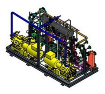
**Project Sibur Portenergo:** Cooling plant for Propane / Butane tank storage 16 Shell and Tube Heat exchangers, 7 vessels (Ø2600x6000), all items assembled in 10 skids (including piping).
