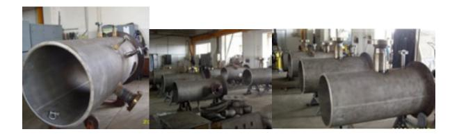
Project Rosneft Propane/Propylene Plant: Gas coolers (Shell and Tube 3,5MW Capacity each) and Separators acc. EN 13445 and GOST
